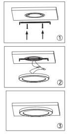
Step1: Fix the installation bracket
