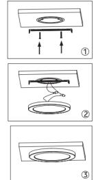
Step1: Fix the installation bracket
