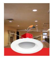
**Description** 5"/6" Round LED Retrofit downlight is engineered with energy-efficient LED technology and with a 120/277V 0-10V dimmable driver for a budget friendly for 0-10V solution. Spun aluminum construction provides clean sharp edges and is suitable for use with most 5" or 6" recessed housings.
