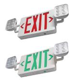
**Description** Self-diagnostic universal field-selectable single/double-face exit light with fully adjustable LED emergency heads. It can be wall or ceiling mounted and suitable for damp locations.
