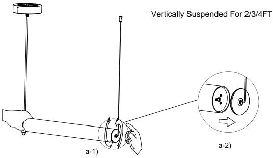
A.Hold the housing with one hand and unscrew the end cap with the aircraft cable using the other hand.
