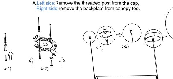
B.Left side: Secure the threaded post using anchor and screws.
