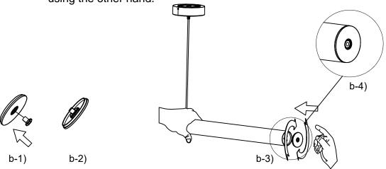
B.Install the screw into the end cap,hold the housing with one hand and screw the end cap into the housing with the other hand.
